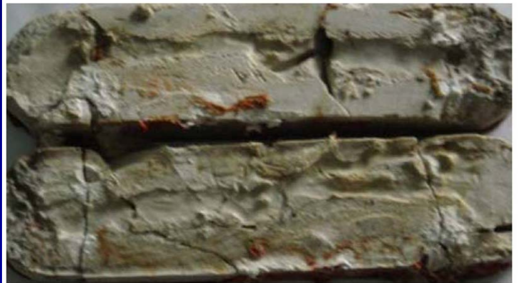
Core picture of acid etched fracture conductivity test
